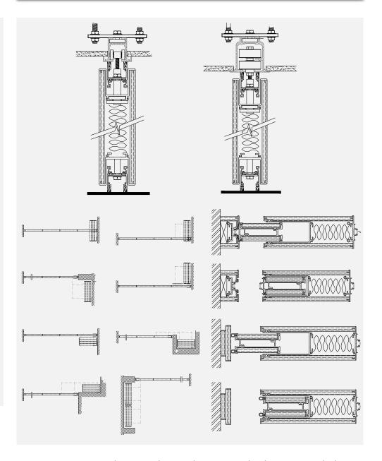
Apton Autonomous is the smart choice, when you need to keep pace with changing space requirements. It is supplied with top hung elements that move easily and quietly in an aluminium track, in either single or twin point suspension.
