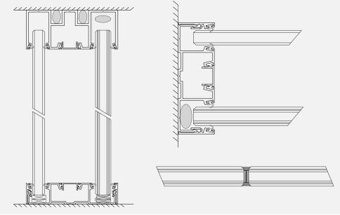
The Quartz frameless glazing system is both stylish and simple. It is mullion free, with minimal tracks at head, base and abutments. 16.8mm FR30/30 glass provides the fire resistance, combined if required in double glazed format, with toughened or laminated glass of thickness 10mm to 19mm. Quartz provides a visually frameless aesthetic with high levels of performance. European fire resistance specification 'EI', (Integrity & insulation).
